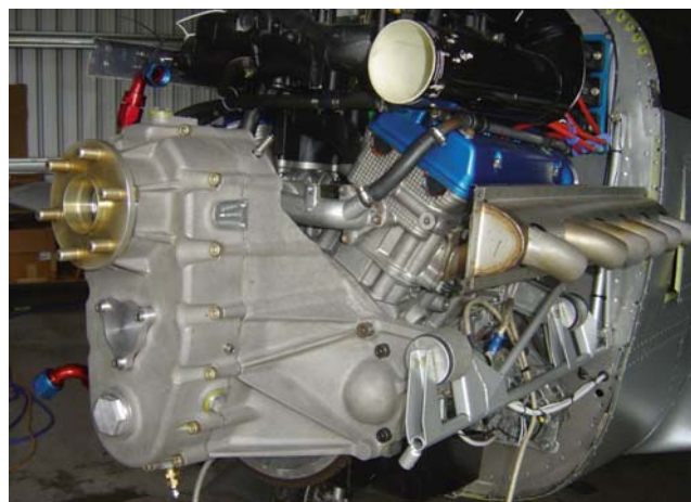
The aircraft is a work of art and so is the gear reduction drive which weighed 3.5kg less than the belt drive unit it replaced.
