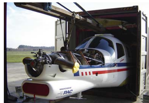
Clearances were barely inches in any given direction. Note the wings already loaded above the fuselage.
