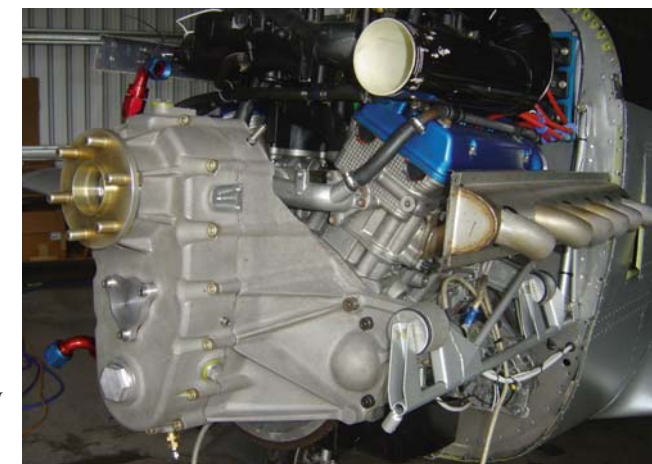
The aircraft is a work of art and so is the gear reduction drive which weighed 3.5kg less than the belt drive unit it replaced.
