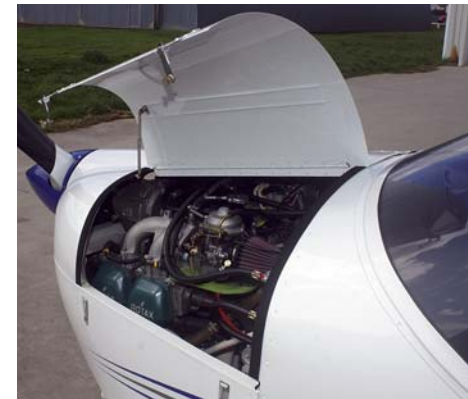
Engine cowls hinge upwards, making for much easier access for coolant checks and pre-flights.
