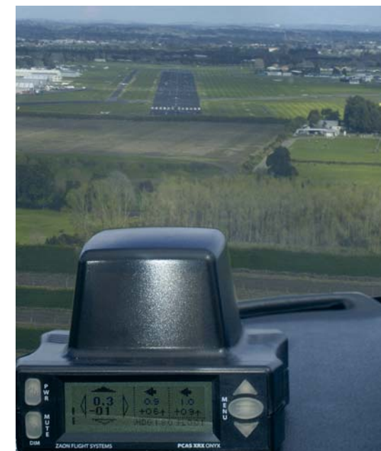
Zaon PCAS operating in stand alone mode on approach to Ardmore. The display indicates nearest traffic on the taxiway 0.3nm ahead and 100' below as well as two aircraft (both recently climbing) in the circuit to our left at relative altitudes of 600' and 900' above.
