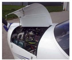
Engine cowls hinge upwards, making for much easier access for coolant checks and pre-flights.
