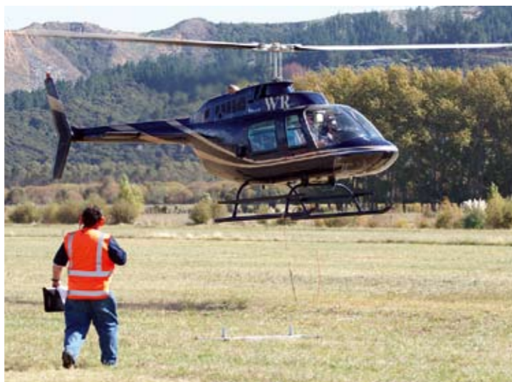
Precision Flying required that one chain (attached to the skids) remained off the ground and the other stayed on the ground, while traversing a marked course.
