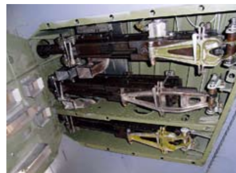
Three guns in place and ready for business. Note the spaces in the hinged panel for spent cartridge shells etc. to fall through.
