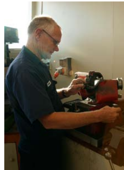
Gary Williams re-facing a rocker in the Aeromotive Cylinder Bay.
