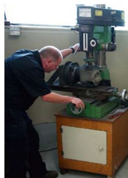
Brett Puddle setting up for port re-facing.
