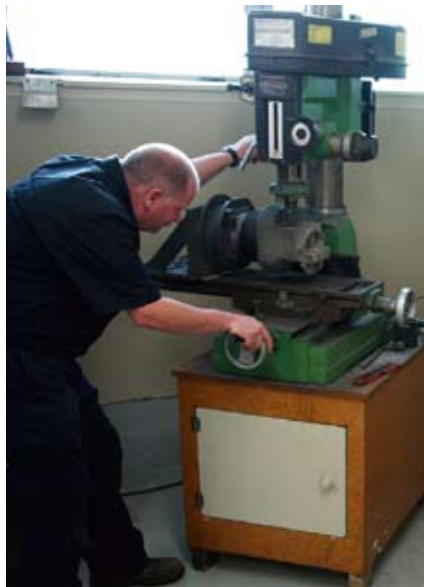
Brett Puddle setting up for port re-facing.
