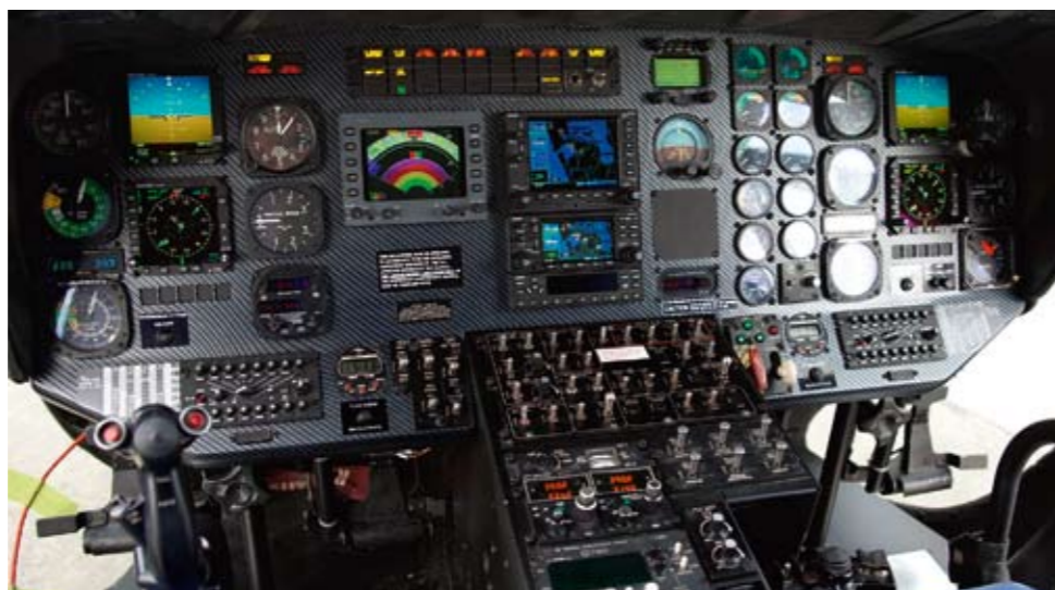
The new panel including EADI, EHSI, AHARS, TAS, GPS and Digital Comms. A H-TAWS is yet to be fitted.
