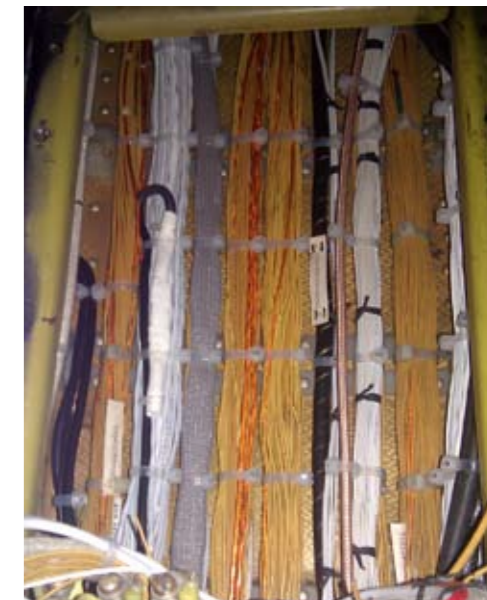
Miles of new wiring were installed, though the aircraft was 50lb lighter once finished.
