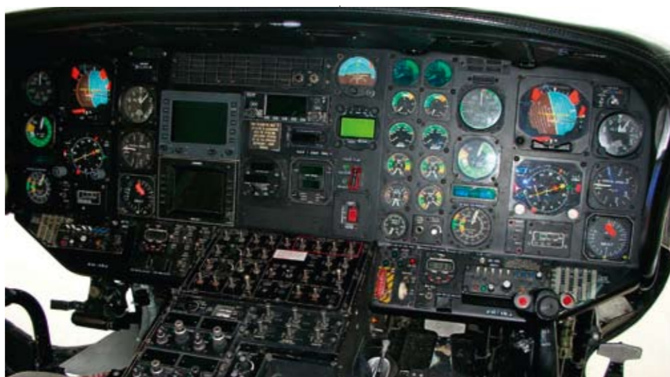
The old instrument panel was full of dated analogue instruments that were becoming expensive to maintain.
