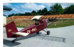
Rod has also used a Chevrolet Corvair engine which he built up himself as per the William Wynne conversion manual and constructed his own propeller to do the initial static engine tests, but has now fitted a 68x32 propeller from Brent Thompson, of Rangiora.
