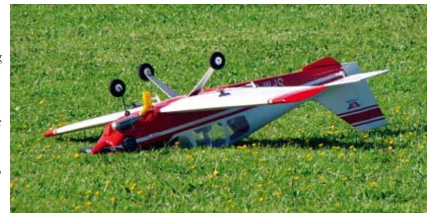
The backward flip. A result of the wind catching under the wing while taxiing.
