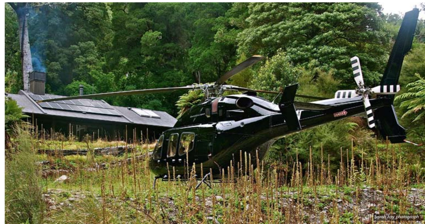
The first Bell 429 for NZ is operated by Advanced Flight on behalf of private owners. Note the tail rotor blades set at uneven intervals to help reduce noise.
