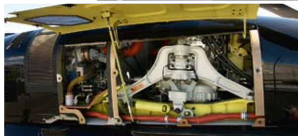
From top: 1. A very elegant panel includes 3 Multi Function Displays; 2. The cabin has hinged and sliding doors on each side for a 1.58m wide opening; 3. Pilot Tony Milligan and the 429 at Auckland Heliport; 4. A cavernous luggage space holds 74 cubic feet or 540lb; 5. Five standard seats (the sixth has been removed) in this cabin configuration; 6. The main rotor transmission is rated to 1100shp and has live mount vibration dampers. The yellow beams underneath run the length of the cabin, forming part of a passenger safety capsule.
