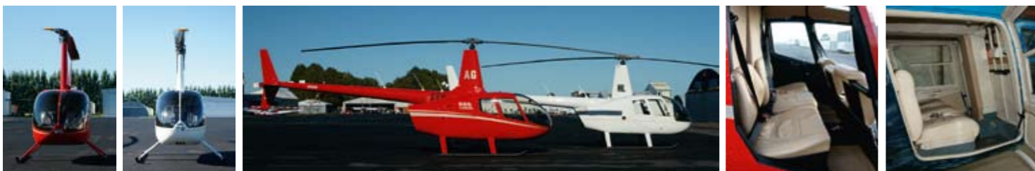
The R66 is virtually identical in length to its R44 sibling. The big difference is an extra 7.5 inches of width, providing significantly more shoulder room up front and of course, space for a fifth seat in the back. Leg room gains an extra inch over the R44. Cabin layout is the same, with an uninterrupted view for rear passengers.
