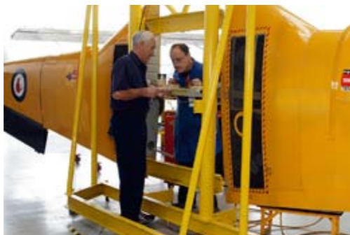
Top: Plenty of variety on the day KiwiFlyer visited. Above: Re-splicing a CT-4 wing for the RNZAF.
