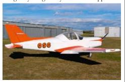
Vidor and went on to become the Alpi Pioneer 300, but the Champion 5 is a plans built wood and fabric version. This is the first of its type for New Zealand (due to being plans built). Grahame has used a Hirth F30U, 92 hp, 4 cylinder 2 stroke engine with a constant speed IVO propeller. The aircraft has a retractable tricycle undercarriage and a roomy cockpit with excellent visibility.
