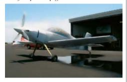
the Czech's own tapered wing design with built in twist and Fowler flaps. This new wing is used on FIZ. The kit which is no longer in production, (being a victim of the USD/Czech exchange rate), was only available as a quick build kit having extensive work done in Texas before shipment to NZ. Final assembly was completed by a team in Gore under the watchful eye of engineer Peter Kempthorne, ensuring CAA requirements were met.
