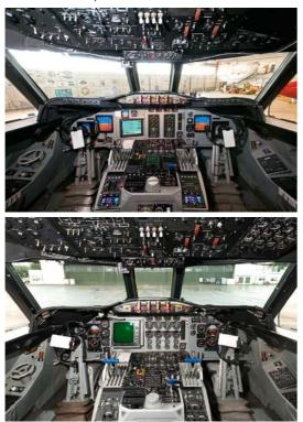
The digital glass cockpit of the new P-3K2 (upper) is a massive improvement on the analogue technology of the legacy aircraft (lower).
