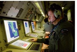
Warrant Officer Rod Simpson operates one of the new tactical crew workstations. Each station is able to operate any of the aircrafts systems to allow maximum flexibility and redundancy. Photo: LAC Grant Armishaw NZDF.
