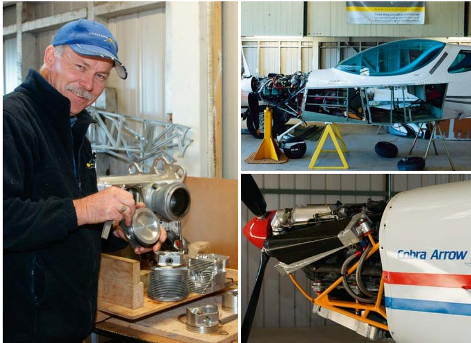
*Clockwise from left: 1) Paul working on a top overhaul of a Jabiru engine, 2) SportCruiser repair project, 3) A new engine frame for an RX8 engine in a Cobra Arrow currently being re-commissioned.*
