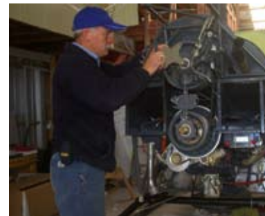
Paul Waterhouse making progress on a well advanced R44 2200 hour rebuild.
