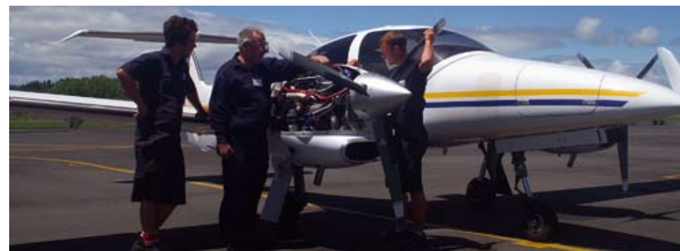
Aeromotive CTC Service Manager, Ross Ward (centre) with trainee engineers and one of eight DA42's under Aeromotive's care. A major current project is their conversion from 1.7 to 2.0 litre engines.
