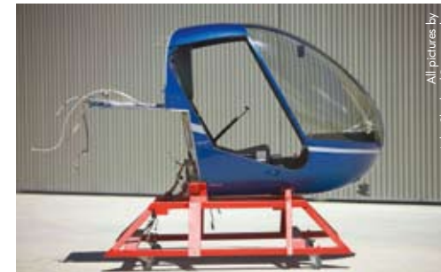
A stripped R22 awaits re-assembly on an overhaul jig.
