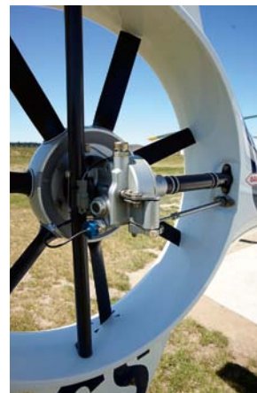
Fenestron control is by cable.
