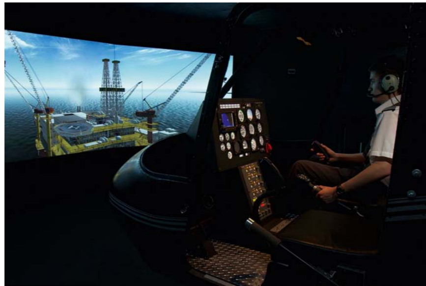
In the 206FX Simulator at Helicopter Flight Training. CAA approved for 20hrs of instrument training time towards an IFR qualification, the sim also provides a safe and efficient means of instilling good habits and training pilots to recover from difficult and high risk situations.
