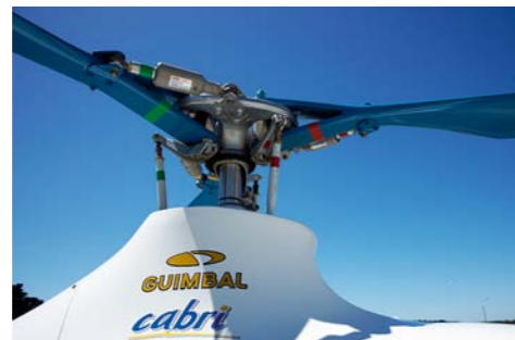
Spheriflex rotor head. Note the blade attachment forks integrated into the composite blades.
