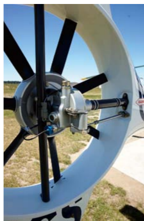
Fenestron control is by cable.
