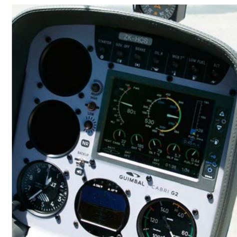
The Electronic Pilot Monitor with automatic display of power available and throttle position, plus fuel burn and flight time remaining.
