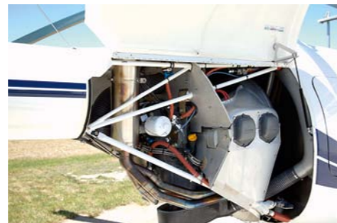
Engine access is very easy. Note the unobstructed oil filler and 4 into 1 inconel exhaust system.
