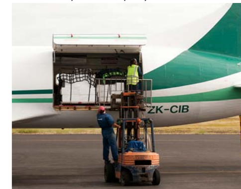
The large side cargo door and roller floor facilitate easy loading of palletised cargo.
