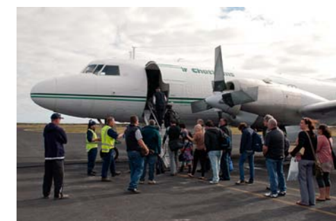
The Convair 580 can carry up to 31 passengers or 6.5 tons of freight depending on configuration.
