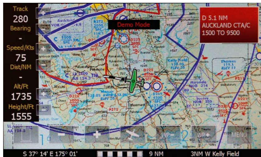
The Clarity 2 screen shown full size. The warning is for the airspace highlighted in red. A line in front of the aircraft indicates 1 minute intervals. Note also the position report bottom right of screen. Menu buttons can be de-cluttered easily if required.
