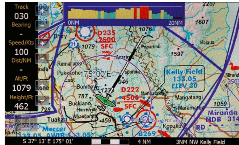
This image (Clarity 2 full size) shows the terrain profile warning in action as well as a 5 mile circle around the aircraft, useful for interpreting distances and map scale. The blue airspace lines show that warnings for this airspace will be activated if appropriate.
