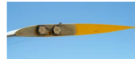
Main rotor blade profile.
