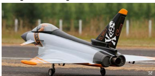
50 lbs of thrust complete with thrust vectoring nozzle.
