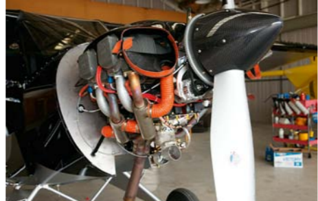
180hp ECi engine in the Carbon Cub SS.
