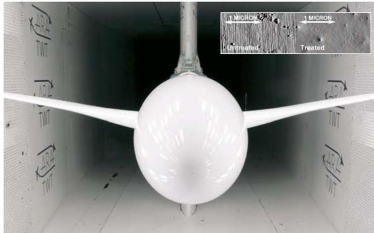
Tested in the Aircraft Research Association's transonic wind tunnel, AGLaze has been proven to reduce drag even on brand new unweathered paint finishes.
