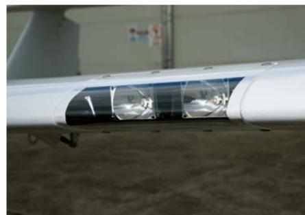
High intensity lights are incorporated on the port side wing.
