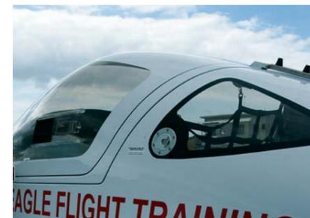
Fueling is straight forward with easy access. The single tank is in the aft fuselage.
