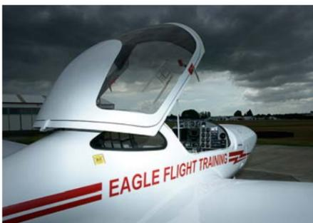
After releasing a latch on each side, the canopy easily lifts on struts to provide excellent access.
