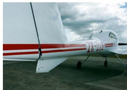
Tail bump protection is provided by a skid with replaceable wear strip.
