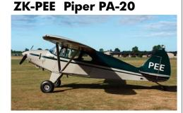
THE PA-20 Pacer is essentially a fourplace version of the two-place PA-17 Vagabond light aircraft, part of the family of strut braced, high-wing light aircraft that were built by Piper Aircraft in the post-World War II period..
