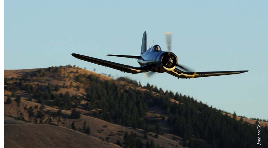
Easily recognised by its wing shape (designed in part to keep the landing gear short and robust for carrier landings), New Zealand's only Goodyear FG-1D Corsair was flown by Keith Skilling.
