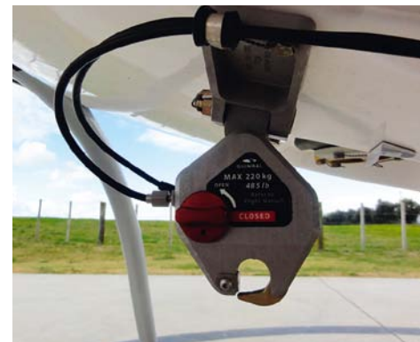
The hook installation. As with the rest of the helicopter, it's an elegant piece of engineering.
