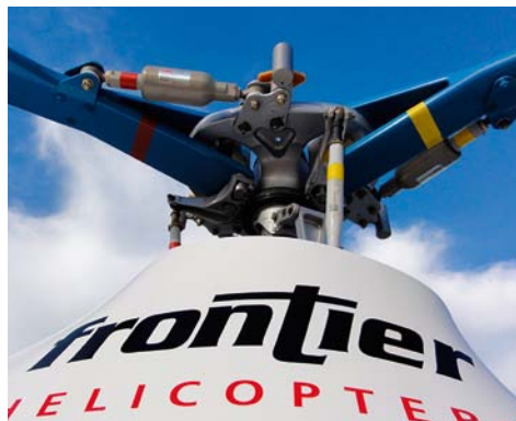
The attachment to the right of the elastomeric damper is the new Vibration Absorbing Pendulum.
