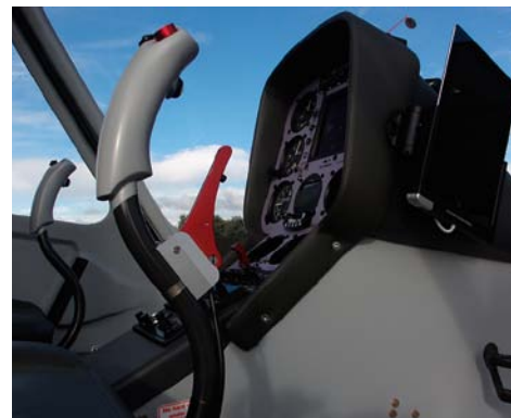
The hook releases are nicely engineered and designed to avoid inadvertent operation.
