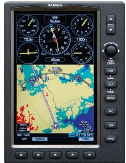
The 695 is robust and elegant. Controls include short cut and soft keys plus a rotary joystick.
