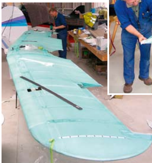
Colin Sutherland reinforces the wing tip area prior to applying further fill and finish coats of butyrate dope.
