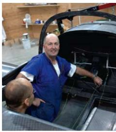
Neil (centre) and Lapo in the Furio fuselage setting up the alignment of rudder cable fittings.
