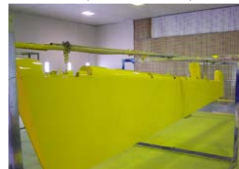
Airspray can also paint or touch-up microlights, helicopters, and in this case a 737 rudder.
