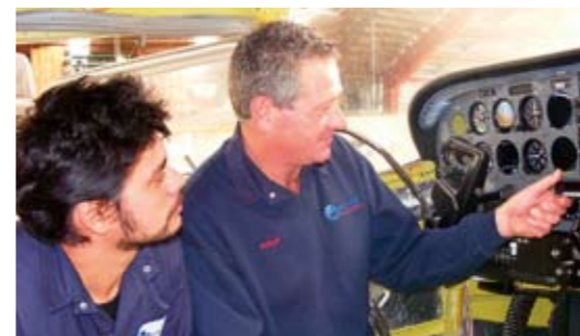
Phil discusses a Cessna 172 radio installation characteristic with Sammy. A full panel rebuild for this aircraft was undertaken in the Aeromotive workshop.
