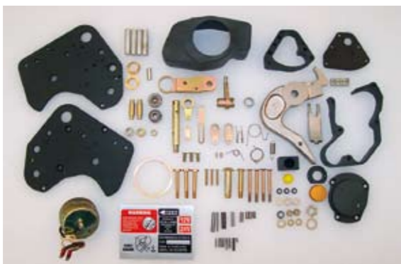
Above: a stripped Breeze Eastern 2A20B hook. At right: On Board Systems Big Mouth, Keeperless and Talon LC hooks ready for despatch
