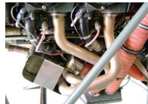
The tidy PowerFlow installation utilises existing hoses.
