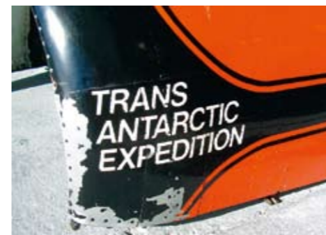
There was plenty of wear and tear on the existing paint scheme
