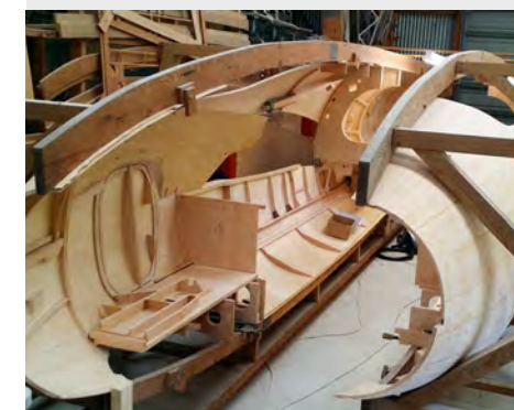
The fuselage is built in two halves and then joined.
