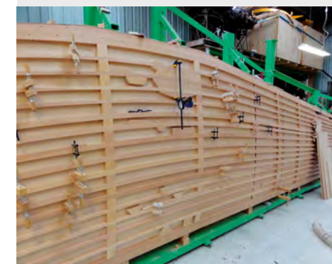
The complex wooden wing is built as one section.
