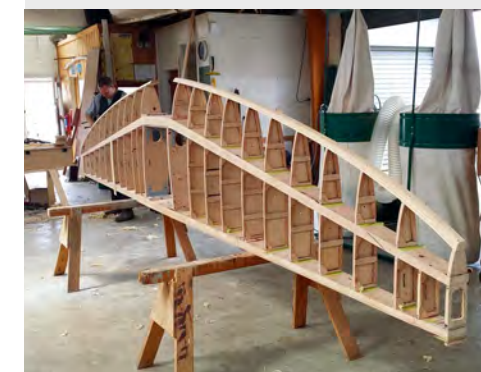
Horizontal tail section under construction.
