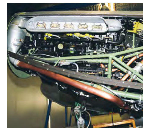
Merlin engine fit out underway. The new sets of Mosquito exhaust stacks are now produced in NZ.
