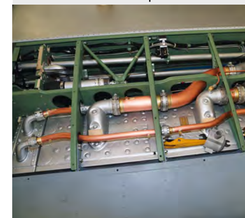
View from on top of the wing looking at the newly built radiators made in New Zealand by Replicore.
