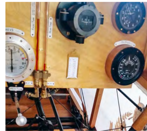
Basic instruments. Note fuel gauge tubes.
