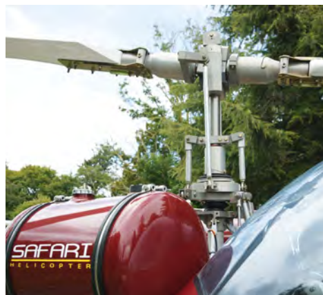
Main rotor blades are composite, made in the US.
