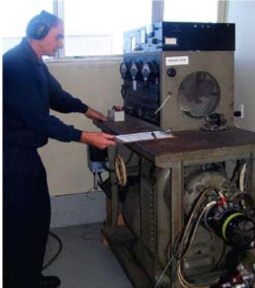
*'Chuck' Osborne at work in the Aeromotive Electrical Bay: Running up a freshly overhauled generator (above) and making repairs to the circuitry of a rudder trim actuator (below).*
