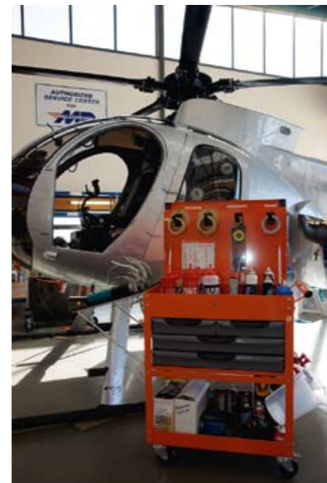
Repeated trips to the consumables store were identified as unnecessary waste. Maintenance trolleys have been set up to avoid this.
