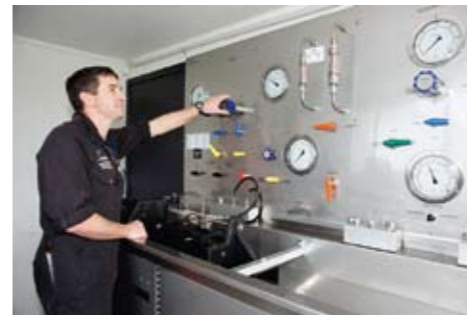
A Dunlop AS350 servo being tested on Oceania's new test rig at Ardmore.
