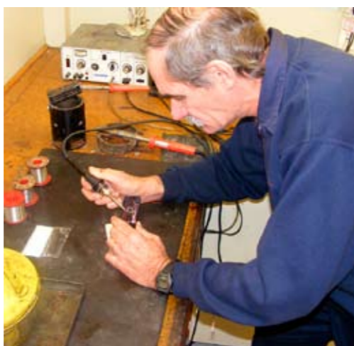
'Chuck' Osborne at work in the Aeromotive Electrical Bay: Running up a freshly overhauled generator (above) and making repairs to the circuitry of a rudder trim actuator (below).
