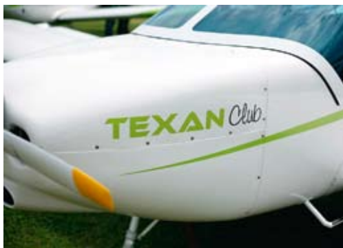
Power is by the ubiquitous 80hp Rotax 912UL fitted with a two bladed wood/composite propeller.
