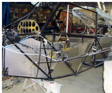
Fabrication and fitting of new interior panels.
