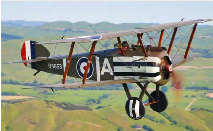
One of the few original Sopwith Camels left flying. It is powered by a Clerget rotary engine and flown by John Lanham.
