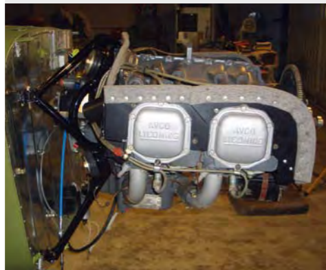
The first fit of the O-360 180 hp engine.
