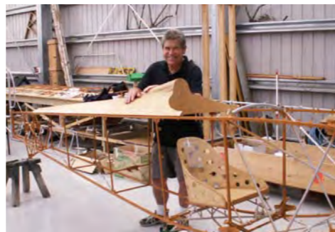
Upper coaming in progress.
