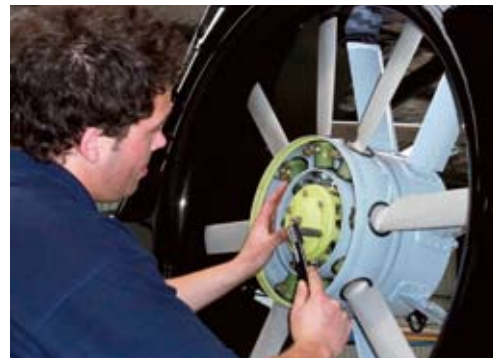
Matt Meyer performing post-inspection assembly of an EC120B fenestron.
