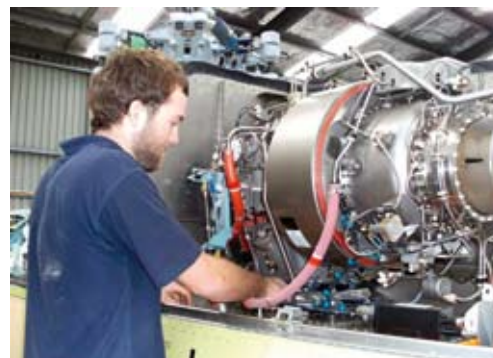
Tom Anselmi conducting scheduled maintenance on an EC120B Arrius 2F engine.
