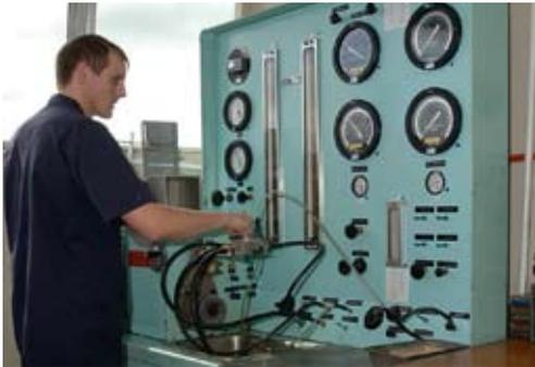
Thomas Kiddle testing the diaphragm section of a RSA7AA1 from a Hughes 300 engine.
