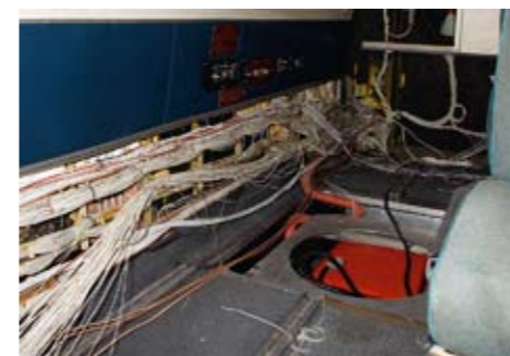
Looking rearward with the cabin partially stripped. Note the camera port in the floor.
