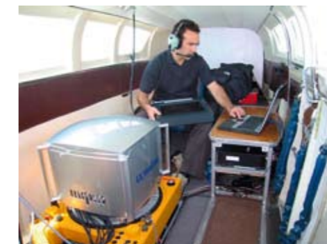
Operating the Vexcel UltraCamX Digital Camera from NZAM's Cessna 402.
