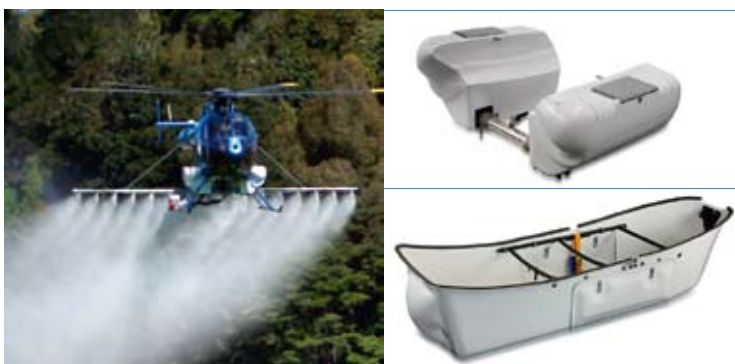
MD500 equipment includes a Spray System and Cargo Pod. Many other products are also available for a variety of helicopter types.
