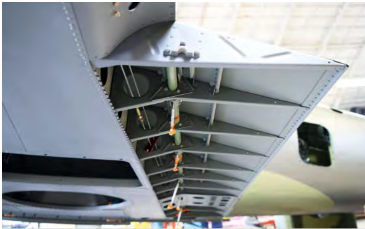
The left wing being prepared for the return of its flaps.
