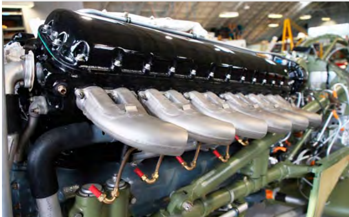
The Allison engine being wired up to run.
