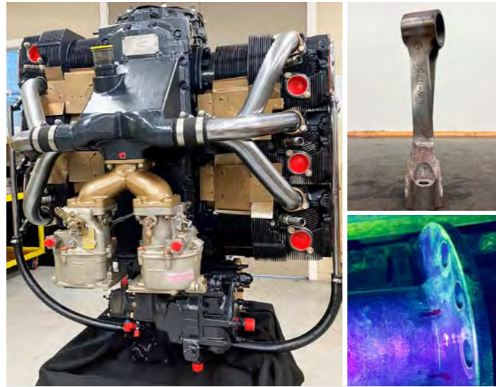
After and before: Freshly overhauled engine, Bent conrod, Cracked flange.
