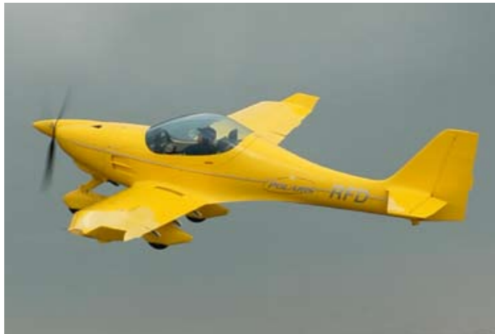
The FK-14 Polaris has electric Fowler flaps which allow wing extension of up to 20%. Powered by a Rotax 912-S, it will cruise at up to 250km/h
