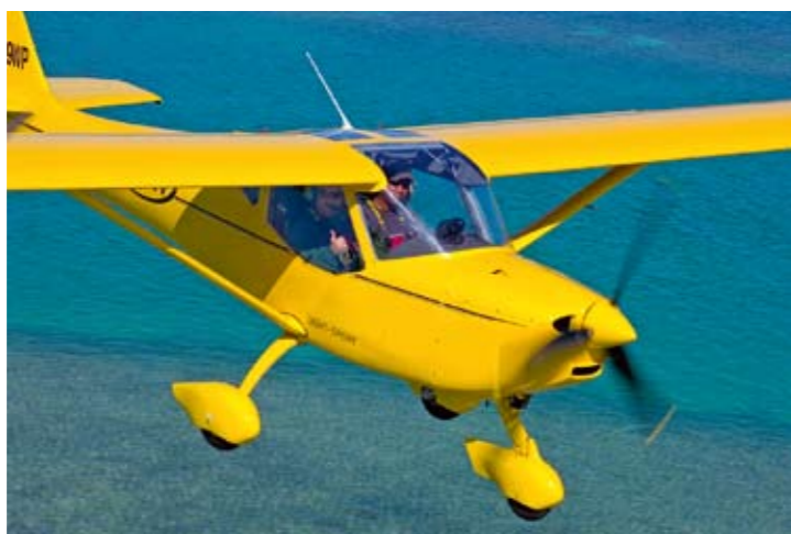
The FK-9 is available in either nose or tail wheel configurations.
