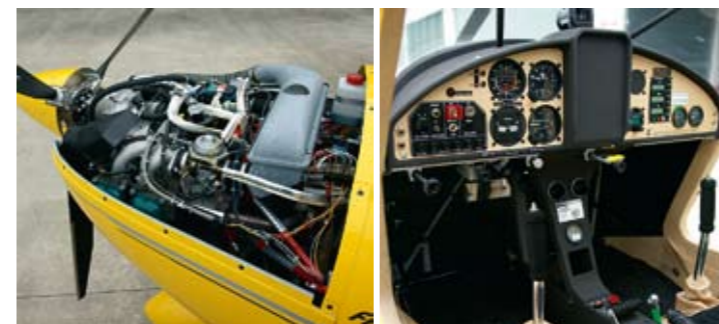
At left: The Rotax 912-S engine installation in the FK-14. At right: Both aircraft have basic instrument panels with plenty of room for expansion.
