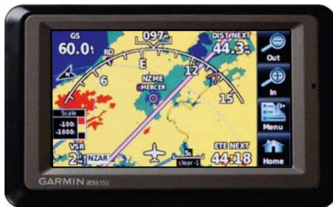
Typical track and route display, in this case with terrain background shading. Points of interest can be selected by touching them on the screen.
