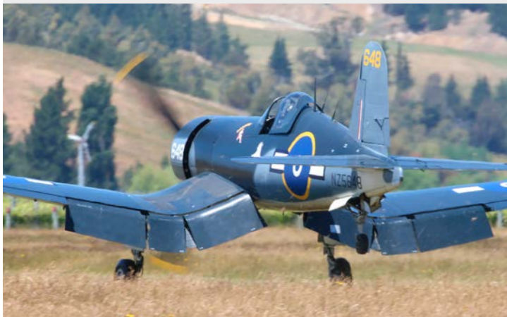
Landing at Omaka after a test flight. The huge flap arrangement can be clearly seen.
