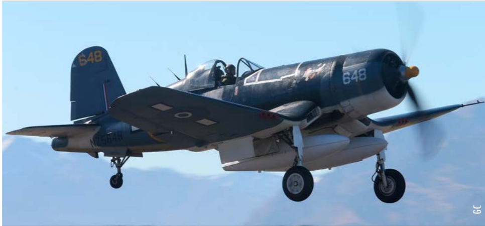
The Corsair roars out of Wanaka with its newly installed long range drop tanks.
