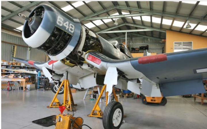
Gear retraction checks being done during the Corsair's annual inspection.
