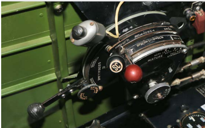
An impressive throttle quadrant. SC stands for supercharger.
